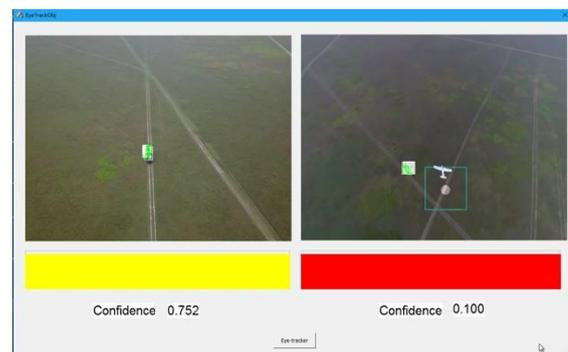
**Figure 1:** An illustration of multi-video surveillance task supported by TLD. The videos were taken by on-board cameras of UAVs. A ground vehicle and an aerial vehicle were being tracked, respectively. In each video stream, the rectangular with feature points (marked in green) indicated the location at which TLD believed the target was. In the right video, the circle (marked in white) indicated the gazing points obtained from the eye-tracker.
