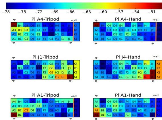
**Figure 4:** Heatmap showing mean RSSI values for the Three Pi's at different positions
